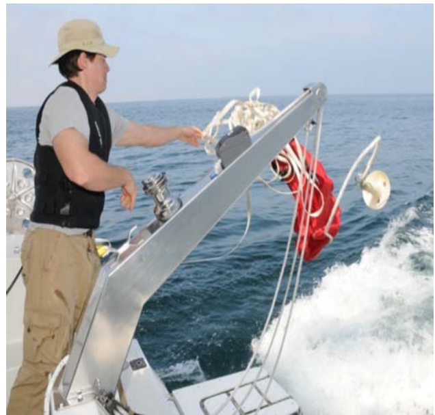
Attach an anchor weight to the "drogue tail." You're now ready to drop the Shark over the lifeline or rail and onto the water. Remember to pay attention to the deployment rode to avoid tangles with your feet.
