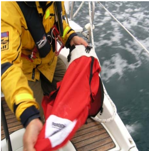
Grab the red canopy inside the Para-Ring and pull it completely out.
